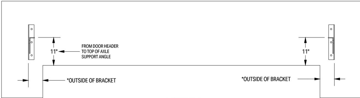
FIGURE 6: DOOR BRACKET TO JAMB
